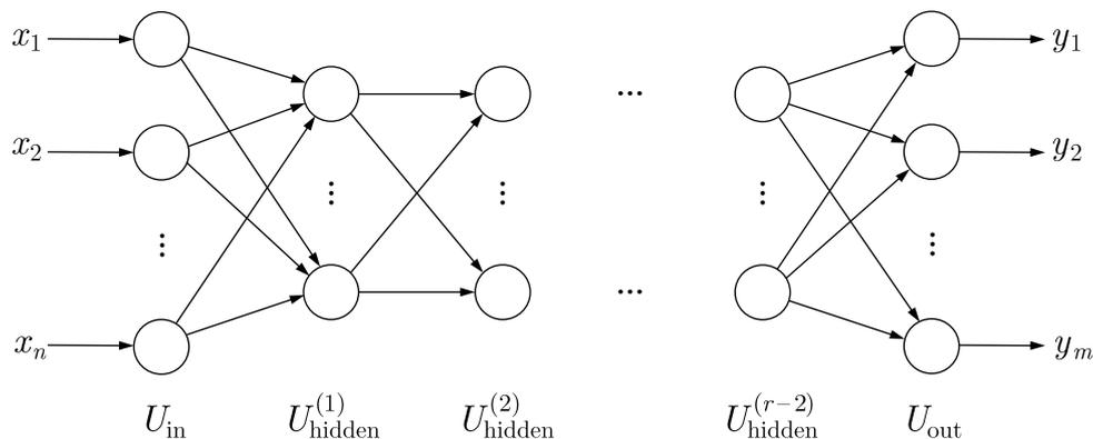
Figure 2.2.: Structure of a  $r$ -layered Perceptron [42, Chapter 5]
