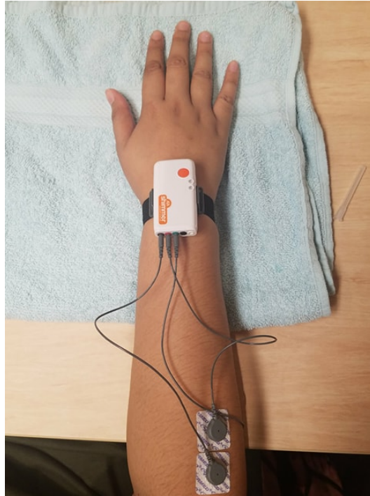
Figure 3.1: The inertial measurement unit attached to the wrist - Cunnington et al. attached the Shimmer 3 device by Realtime technologies ltd to the wrist of the throwing arm to record throw kinematics and muscle activity.
