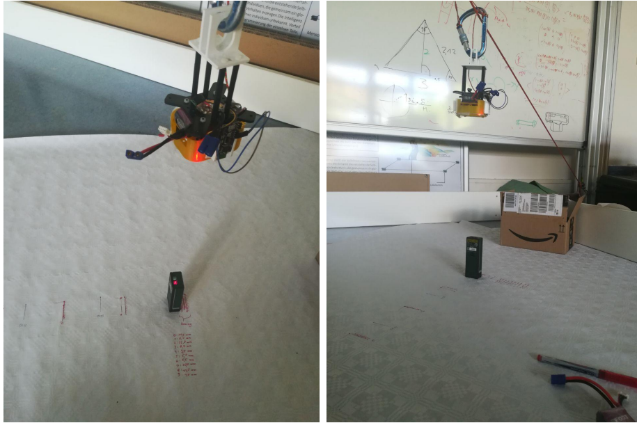
Figure 5.4: Markings on the Ground for the Manual Measured Distances
